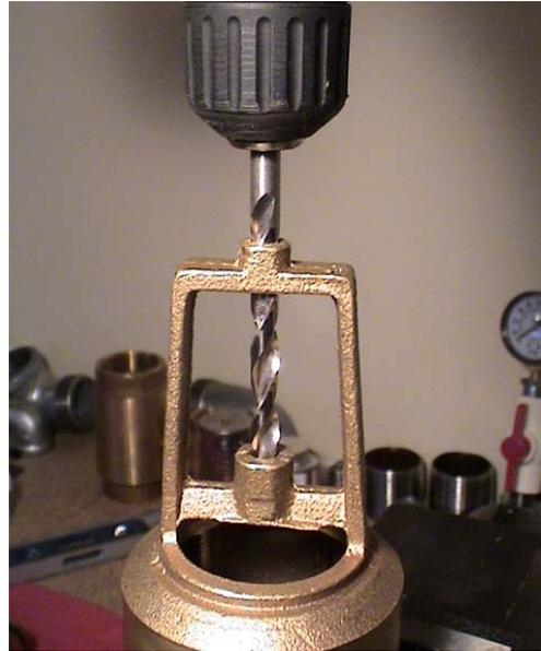
Drilling out to fit the 5/16" hardware
