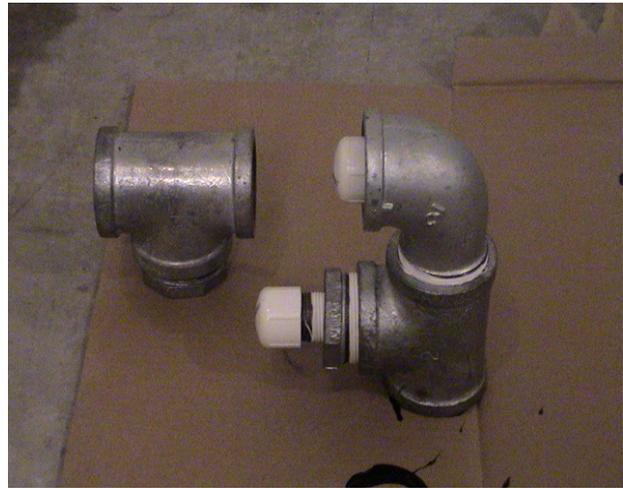
Remove the PVC caps or plugs for good air flow and set aside to let dry.
