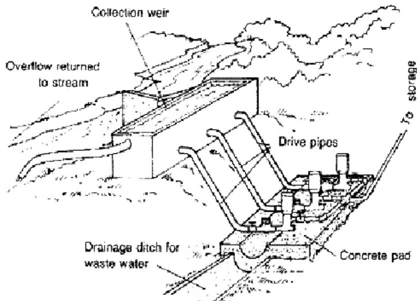
The smaller 1" RAM the HRP1-1 will operate well on around 5 gallons of water flow per minute. The goal of course is to develop your source to provide at least 10 gallons per minute so this is eliminated as a critical factor. Beyond 10 gallons per minute consider moving to the 2" ram designs if you need the higher delivery volumes.
