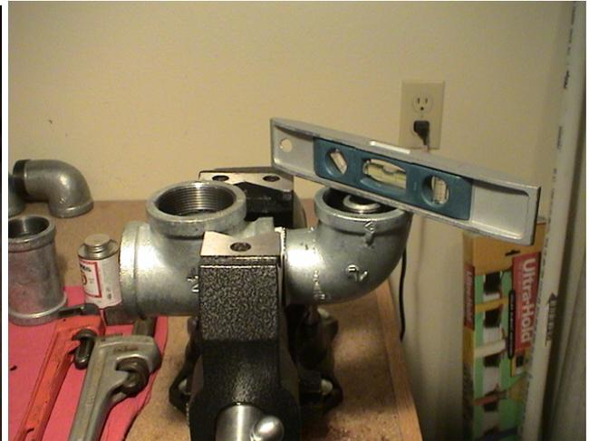
Now get the output "T" ready by installing the bushing.
