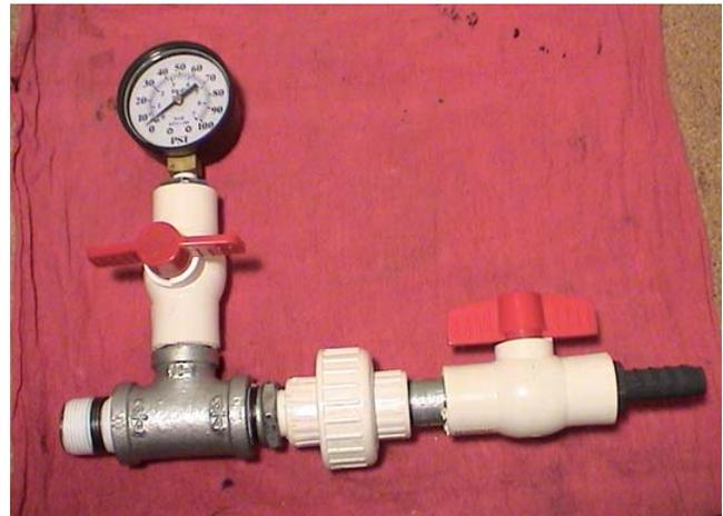
Completed Valve / Gauge Assembly
