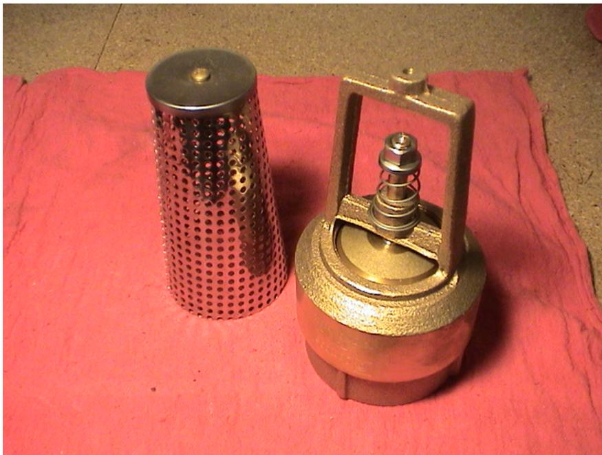
2" Brass Foot Valve with screen removed
