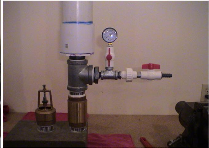
Adding the Pressure Gauge / Ball Valves
