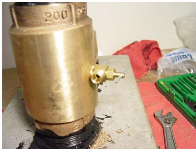
Needle valve installed.
