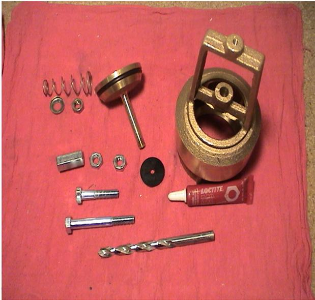
2" Foot Valve disassembled with parts
