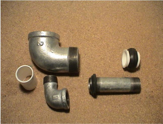
Parts to construct Valve Mount
