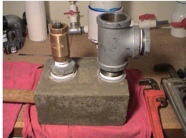
Attaching the "T" with bushing
