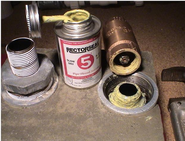
Applying liquid thread sealant
