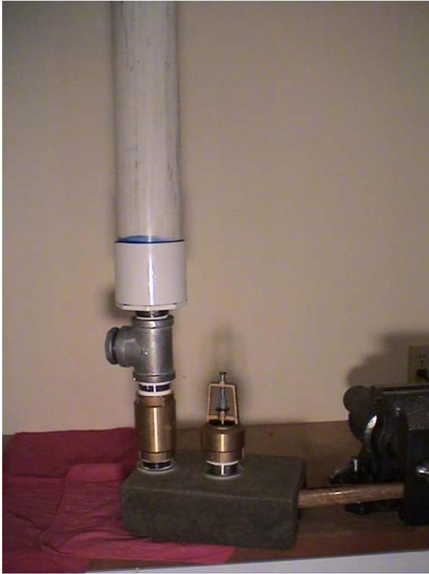
Pressure Chamber Installed
